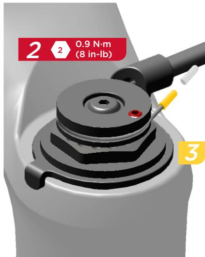
Pull the cable taut, then tighten the bolt to 0.9 N·m (8 in-lb). Cut the cable to length.
