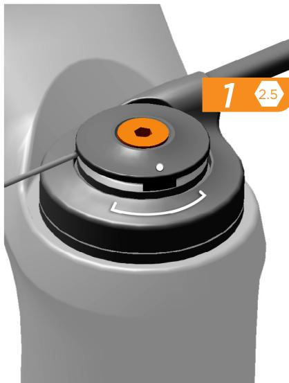
Use a 2.5 mm hex wrench to loosen the cable spool bolt 1/4 turn.
