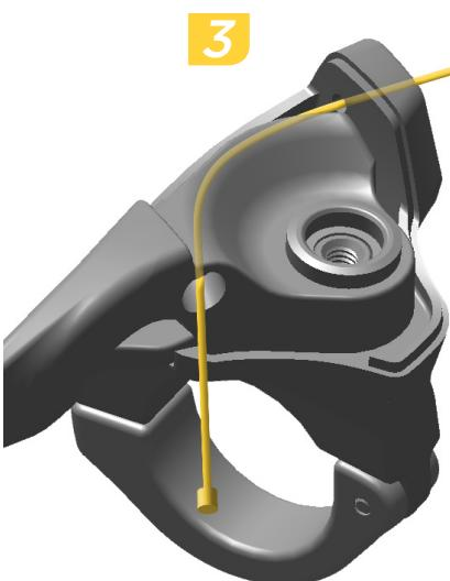
Place your finger over the bolt hole on the lever to prevent the lever from moving, then route the shift cable through the upper cable ports.
