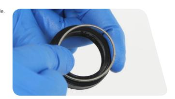
Insert the narrow end of a new wiper seal into the recessed end of the appropriate RockShox® seal installation tool.
