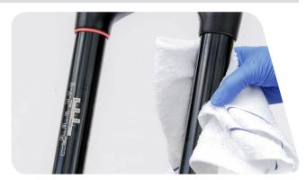
Apply grease to the inner surfaces of the wiper seals.
