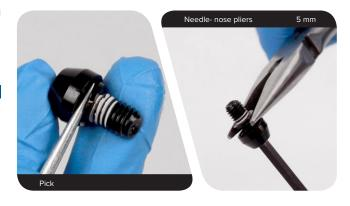
Install the black bottom bolt into the spring side shaft of the lower leg. Install the red bottom bolt into the damper side shaft of the lower leg.
