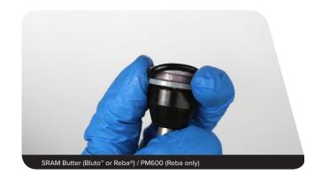
Remove the top out bumper cone from the air piston. Inspect the tension pin hole on the air piston. Install the top out bumper cone onto the air piston.
