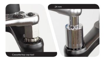
Remove the top cap o-ring. Install a new o-ring. Do not apply grease to the top cap threads.
