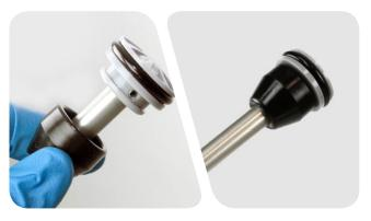
Apply a liberal amount of grease to the inside of the upper tube, from the end of the tube to approximately 60 mm into the tube.
