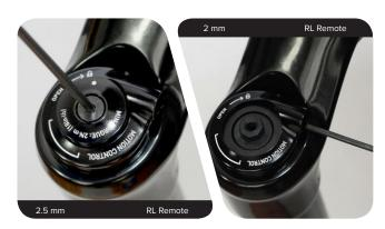
Loosen the compression damper top cap.
