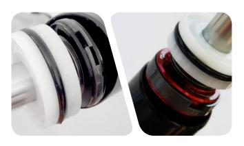
Push the rebound seal head into the upper tube until the retaining ring groove is visible.
