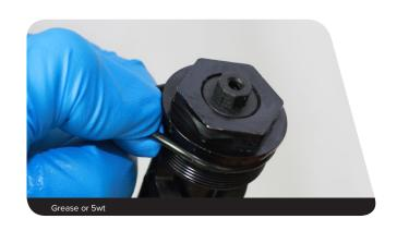
Remove the compression damper piston o-ring. Apply grease to the new o-ring and install it.
