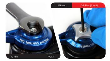
$\mbox{\bf RL:}$  Install the lockout adjuster knob on the top cap so the knob rotates from open to closed.
