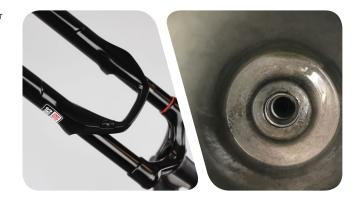
200 hour service only: Use a pick and needle nose pliers to remove the old crush washers from each bottom bolt.
