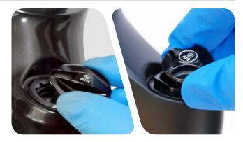
Depress the Schrader valve and release all air pressure.
