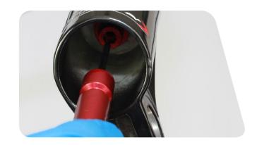
PRefer to your pre-service recorded settings to pressurize your air spring, or use the air chart on the fork's lower leg and pressurize the air spring.
