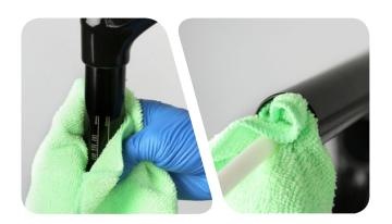
9 Remove the seal head from the rebound damper shaft.
