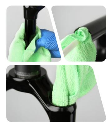
Remove the seal head assembly from the air shaft.
