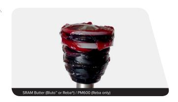
Apply a liberal amount of grease 40-60 mm wide around the air shaft.
