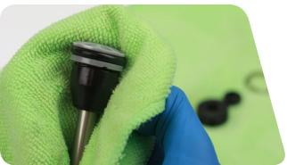
Remove the outer and inner o-rings on the floating seal head. Apply grease and install new o-rings.
