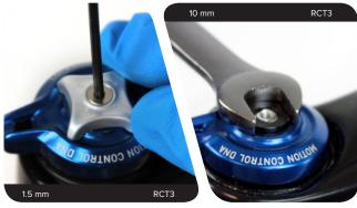
**RL Remote:** Press the remote lever in to the open position. Remove the retention screw, cable spool, and cable. Loosen the remote cable stop collar clamping bolt. Remove the cable stop collar.
