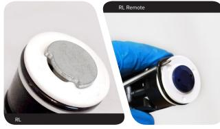
**RCT3:** Install a new glide ring on the compression damper piston.
