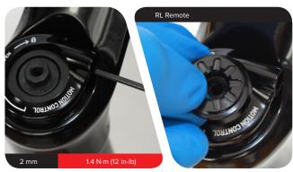
Install the cable spool top so the indicator dot on the cable spool is oriented within the bracket printed on the cable stop. Install and tighten the set screw.
