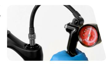
Install the air valve cap onto the air spring top cap.
