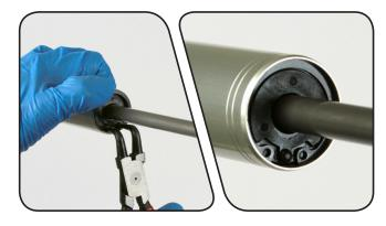
Use a pick to remove the top cap o-ring. Apply a small amount of 12 grease to a new top cap o-ring and install it. Apply a small amount of grease to the top cap threads.
