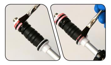
Firmly push the air assembly into the bottom of the upper tube while gently rocking the air shaft side to side.
