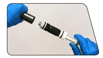
4 Spray isopropyl alcohol on the inside and outside of the air tube and wipe it with a clean rag. Wrap a clean rag around a long dowel and insert it into the air tube to clean inside the air tube.
