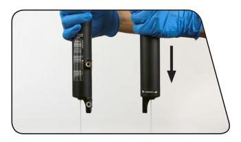
Remove the lower leg from the fork by pulling it downward, holding onto both legs or the brake arch.
