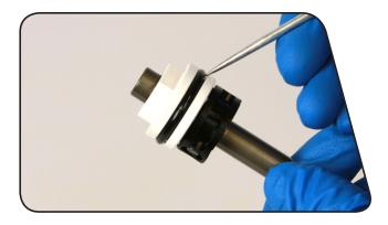
7 Remove the top out bumper from the negative piston. Use a pick to remove the inner and outer negative piston o-rings.
