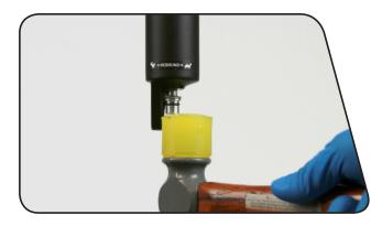
*6* Firmly pull the lower leg downward until oil begins to drain.
