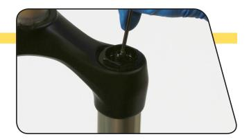
Remove the external rebound adjuster knob by pulling it from the shaft bolt at the bottom of the right fork leg.
