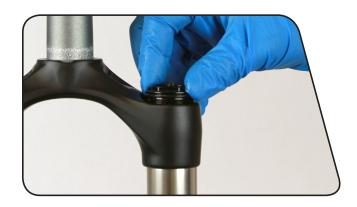
Use a torque wrench and a 24 mm socket to tighten the top cap to 7.3 N·m (65 in-lb).
