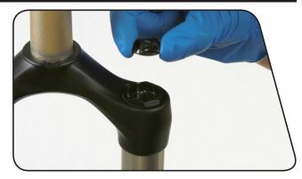
2 Depress the Schrader valve and release all of the air pressure from the air chamber.
