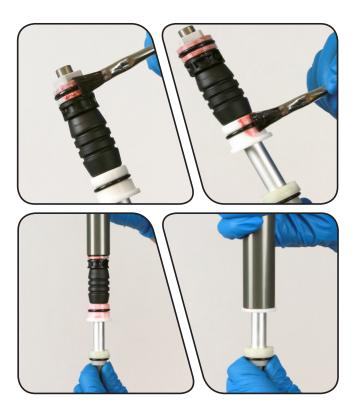
11 Use a pick to remove the top cap o-rings. Apply a small amount of grease to a new top cap o rings a thin to the grease to a new top cap o-rings and install them.
