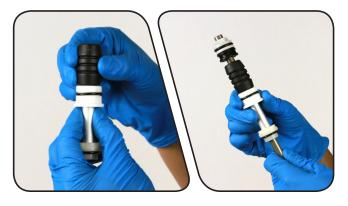
Apply grease to the inside of the air tube, from one end of the tube to approximately 60 mm into the tube.
