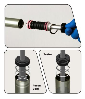
Install the snap ring onto large internal snap ring pliers. Use the pliers to push the base plate internal snap ring pliers. pliers to push the base plate into the upper tube while installing the snap ring into its groove. The base plate tab should be situated between the snap ring eyelets.
