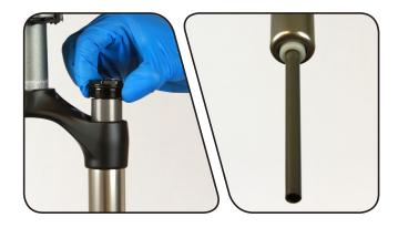
Apply a small amount of grease to the top cap threads and o-ring. Thread the top cap into the upper tube.
