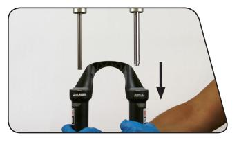
B Spray isopropyl alcohol on and into the lower leg. Wipe the lower legs clean, then wrap a clean rag around a dowel and clean the inside of each lower leg.
