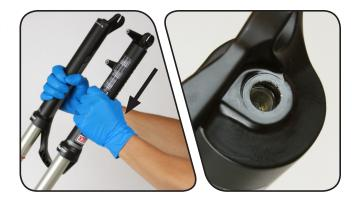
6 Clean the shaft bolts, crush washers, and crush washer retainers. Inspect the crush washers and retainers. If the crush washers or retainers are flattened or deformed, replace them with new ones.
